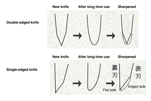
6. As sharpening, an arch may appears on the tip of blade of other side. Lightly sharpen both sides to remove the arch to finish.
